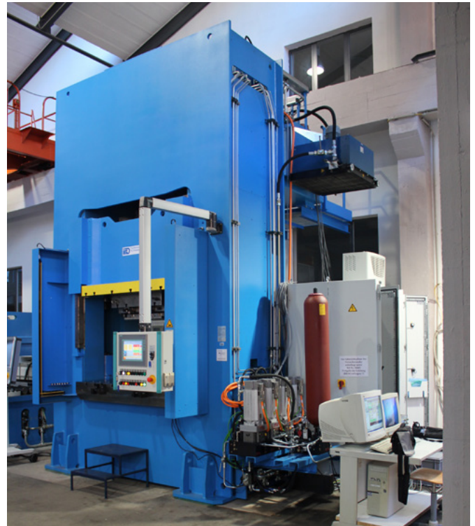
Figure 2: Deep Drawing Press using electro-hydrostatic actuation for the die cushion axis. Source: Dresden University
